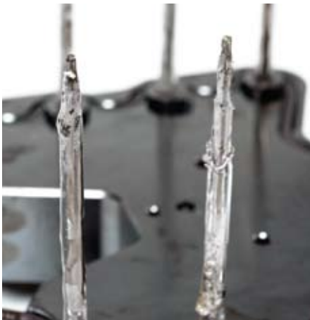
Refurbishment techniques such as fluidized beds restore hot runners to like-new levels.
