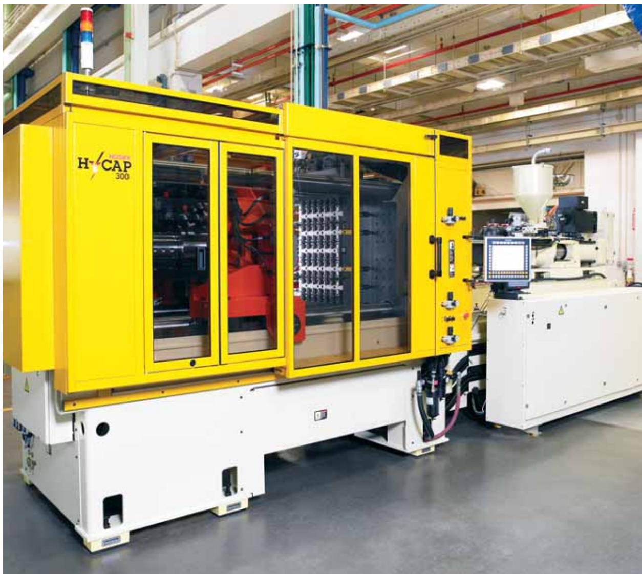
A HyCAP 300 RS65/60, 72-cavity system for lightweight water closures.
